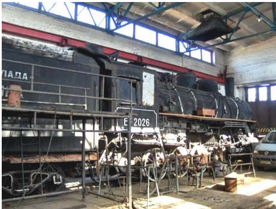
The ALCO 2-10-0 awaiting restoration in the Tsvetkovo workshops. Photo: Ivor Harding
